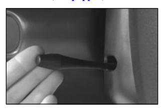
A tilt steering wheel allows you to adjust the steering wheel before you drive. You can also raise it to the highest level to give your legs more room when you exit and enter the vehicle.
